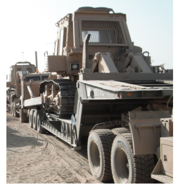
870 trailer loaded with dozer
